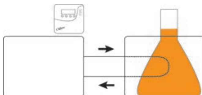
Capable of external circulation in a closed circuit
